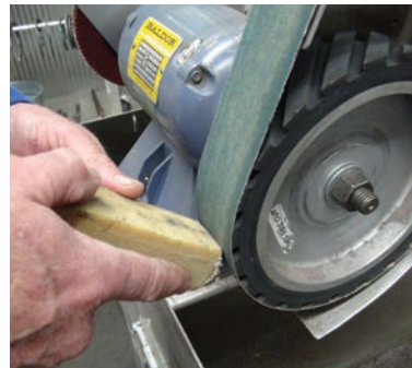
To clean belt, place rubber cleaning stick on belt at a 45° angle.
