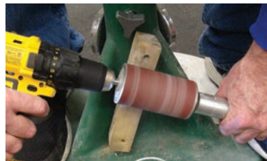
To clean sleeve, hold buffer against rubber stick and run drill. Sweep buffer side-to-side until material is removed. Be sure to set drill direction to ensure rotation is throwing material down and not up.
