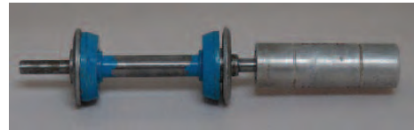
3. Hoof Buffer with bladder removed and ready for new bladder.
