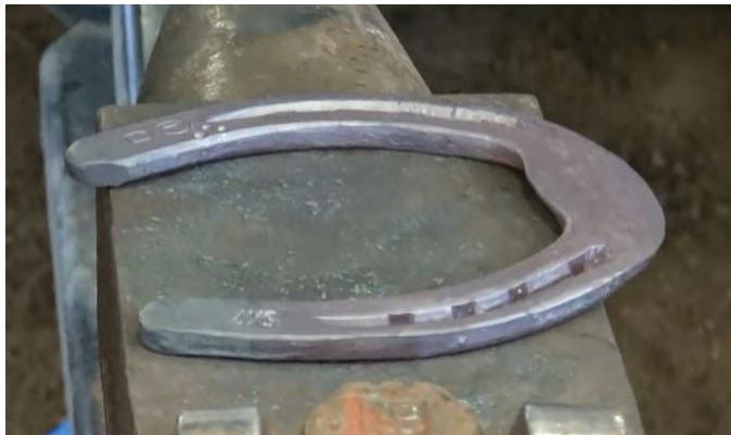
Final forging of the SX-7 on face of anvil.
