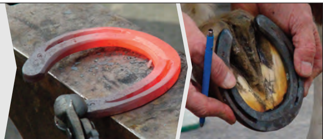
Medial heel ground to allow for sinking in the surface.
