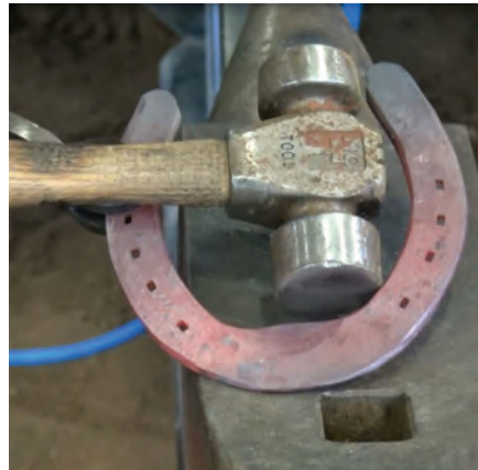
Using an SX-7, you can accomplish a similar result but with less metal you may not get the desired width.
