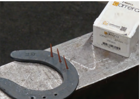
Pride 1-1/4" with Liberty Carrera Nails. The extra "neck" of the Carrera fits securely in the punching.
