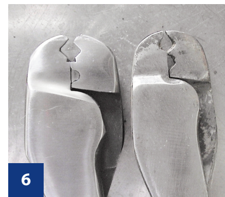
6 Older tool on right has been modified and used properly. Fairly new tool on left with broken tip.
