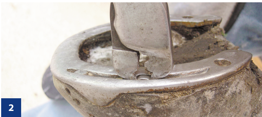
2 Puller tips are not under nail head; this method causes damage to tool.
