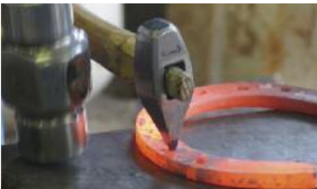
Forepunch to final depth, drift and pritchel.
