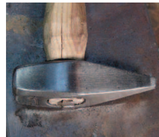
Damaged Wood Handled Forepunch. No heat signature at tip, E-head "wedge" split handle.
