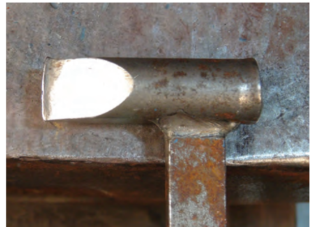
LEFT HANDER USED THIS IN CROSSOVER STYLE. NOTE DAMAGE TO FULLER END.
